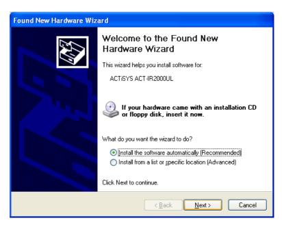
If you kept the CD in the CDROM, Windows XP will automatically search for all drivers compatible with IR2000UL. You will see a window with a choice of different drivers, please select the OEM one. If you install the driver to WindowsXP, the driver will automatically copy to Hard disk (C:\Windows). Please highlight "C:\Windows\inf\oem0.inf" and click "OK" button, the WindowsXP system will automatically install IR2000UL.
